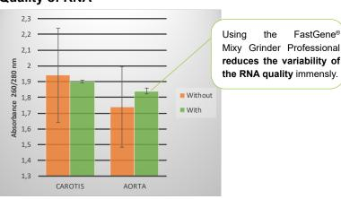
The RNA yield was extensively increased by 6 - 20 fold when using the FastGene® Mixy Grinder Professional. Additionally, the quality of the RNA measured spectrometrically showed considerably less variation when using the FastGene® Mixy Grinder Professional (absorbance at 260/280 nm is 1,94±0,30 without vs 1,90±0,01 with the FastGene® Mixy Grinder Professional).
