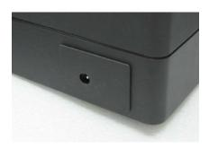
Adaptor input: 12V DC, Power AC input: 100~240 V; 50/60 Hz power source
